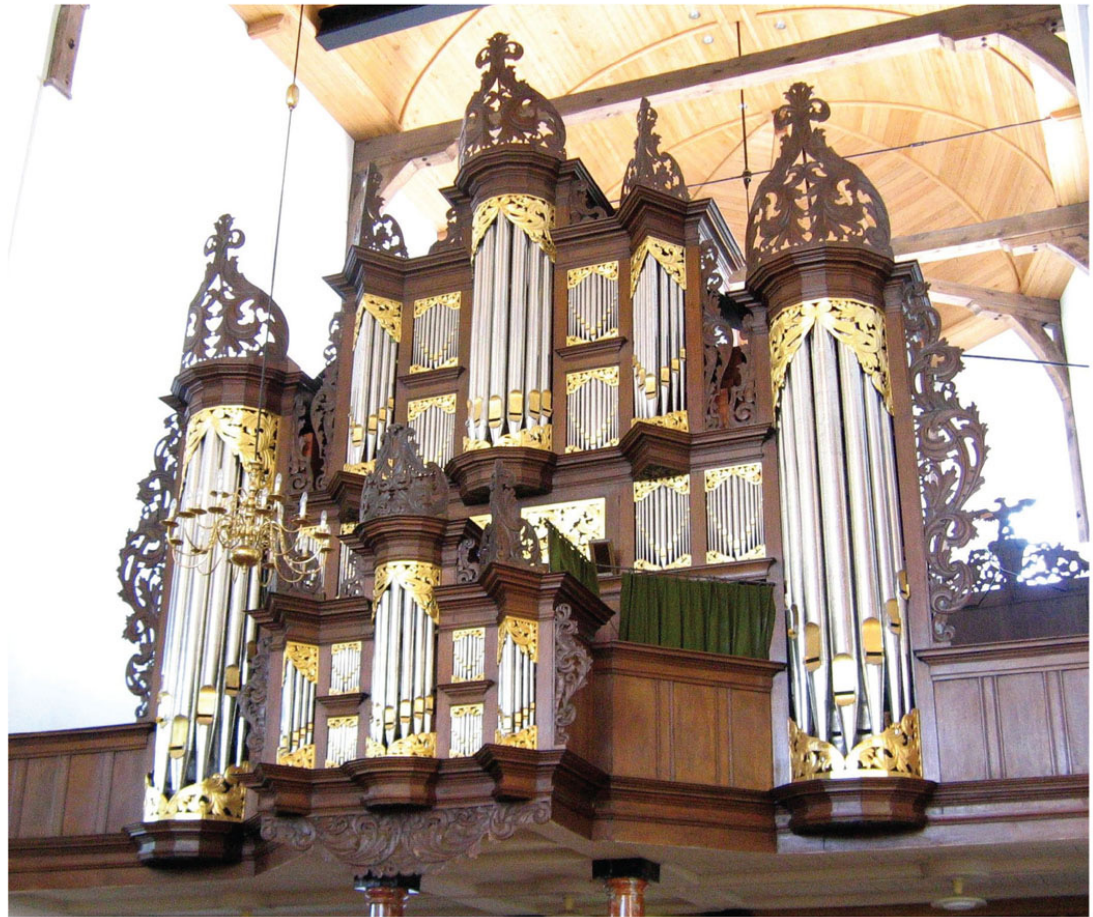
FIGURE 17.10 Organ built in 1710–11 by Arp Schnitger in the Martinikerk in Sneek, a city in the northern Netherlands. The upper chest of pipes is the Hauptwerk, or Great organ. The tall pipes in the center and around the sides produce the lowest notes, played by the pedals. Below the Hauptwerk is the Brustwerk, and below that, unseen in this photograph, are the manual keyboards, the pedal keyboard, and the organist's bench. In the foreground is the Rückpositiv, mounted on the railing behind the organist.
